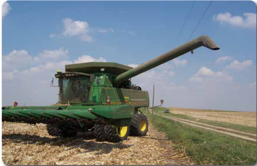
Grain augers coming into contact with overhead power lines is a major hazard during harvest season. Always know your surroundings when farming!
